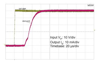
Figure 6: Typical step response (0 to 50 V)
