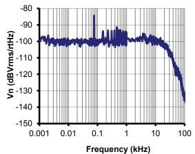
Figure 13: Typical noise voltage density of V ( $R_{\rm M}$ ) with  $R_{\rm M}$  = 50  $\Omega$
