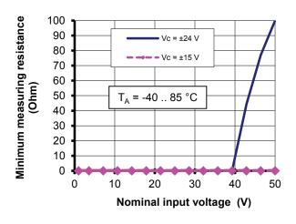
Figure 2: Minimum measuring resistance; For  $\mathbf{T}_{\mathrm{A}}$  under 80°C, the minimum measuring resistance is 0  $\Omega$  whatever  $\mathbf{V}_{\mathrm{C}}$
