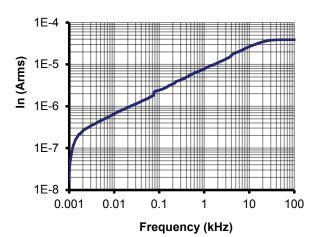
Figure 14: Typical total output current noise (rms) with  $R_{\rm M}$  = 50  $\Omega$  (fc is upper cut-off frequency of bandpass, low cut off frequency is 1 Hz)
