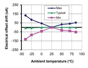
Figure 3: Electrical offset thermal drift
