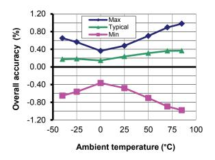
Figure 4: Overall accuracy in temperature
