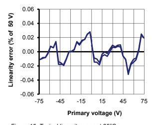
Figure 15: Typical linearity error at 25°C
