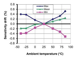
Figure 5: Sensitivity thermal drift
