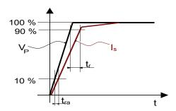
Figure 17: response time  $t_r$  and reaction time  $t_{ra}$
