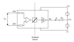
standard characterization schematics for current output transducers ( $R_{\rm M}$  = 50  $\Omega$  unless otherwise noted)
