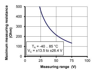
Figure 1: Maximum measuring resistance
